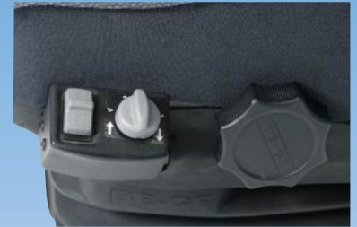
Control panel for quick lowering and stepless height adjustment.
